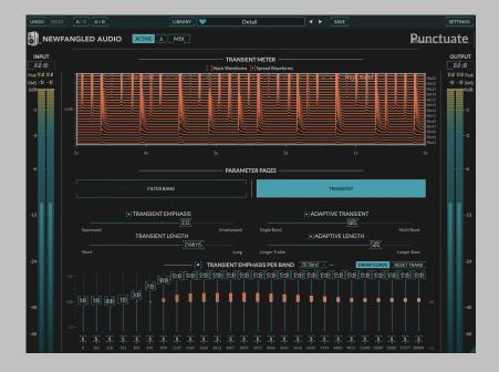
Punctuate is heavily based on the Transient Emphasis section of the Elevate Mastering Limiter. It is a multi-band transient modulator (sometimes called a transient designer) that uses, by default, the 26 critical bands in the human ear. In addition to using the critical bands it uses intelligent algorithms to set the parameters of the transient modulator for each band. This allows you to control the transient emphasis (or suppression) and timing across all 26 bands with just 4 controls.
